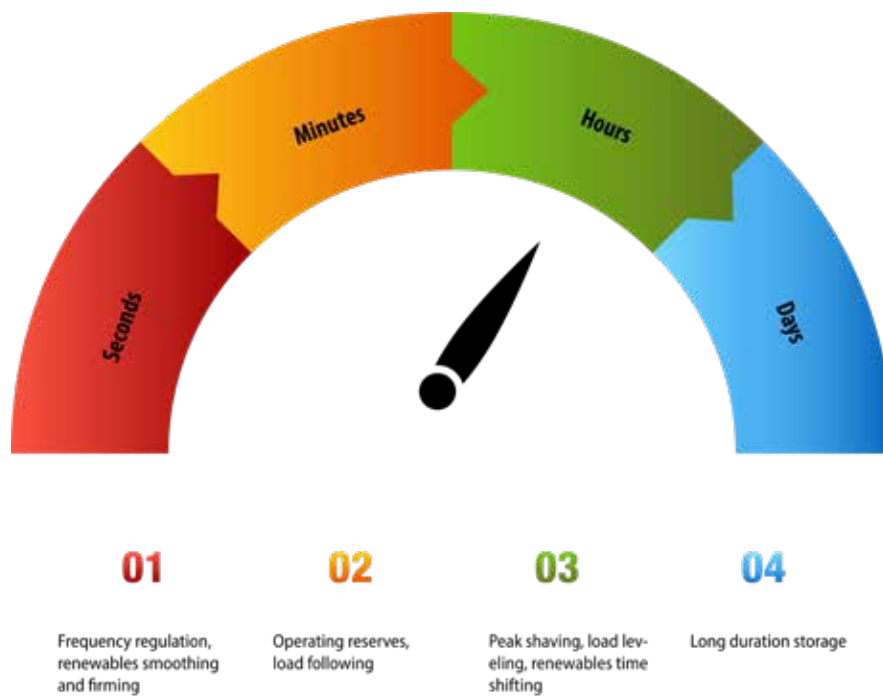
Figure 13.4-5: Battery Energy Storage Applications
